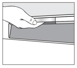
Reach under the handle and pull the door open.
